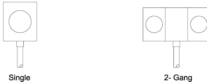
Meter Sockets-Single and Duplex Note C
